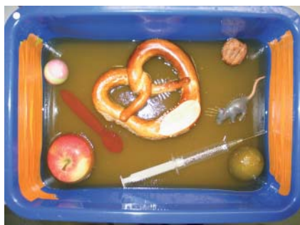
Fig. 1 Plastic box with different objects after casting in the first layer of agar: rubber ball, pretzel, walnut, plastic spoon, apple, syringe, plastic mouse, lime.
