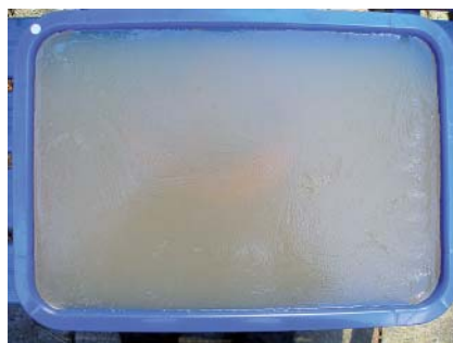
Fig. 2 Plastic box was filled with agar. After hardening of the last layer, the objects were no longer visible.
