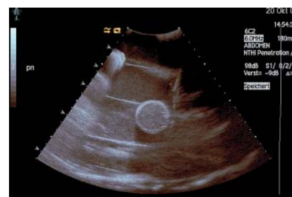
Fig. 4 Visualization of a rubber ball in the plastic box filled with agar.
